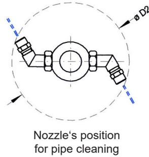
1. With **smooth jet nozzles** equipped as **dirt cutter**. Parts driven by are cleaned with maximum force of impact.
