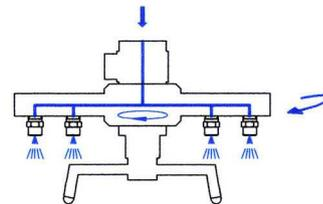
2. Rinsing resp. blowing-off - max. 50 l/min. - max. 10 bar
