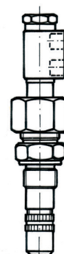
Nozzle lance, clamping and height adjustment via a clamping ring screw connection, with head thread, suitable for ZL 3/8" and ZL 1/2" lance-Ø
