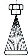
Square impact area, up to 50° spray angle is marked with an E; e.g. FL E 30-20, available on request
